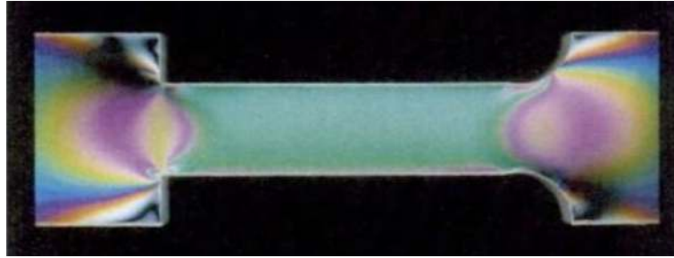
Figure 3.25: Influence of a connecting fillet on a tensile specimen: photoelastic observations (isochromatic fringes).
