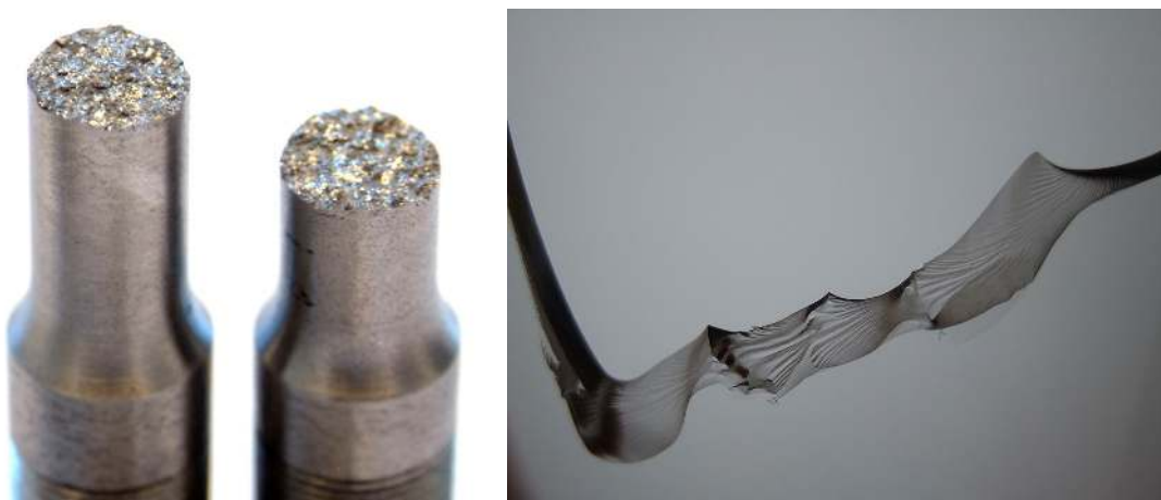
Figure 3.7: Fracture surfaces in the case of cast iron (left) and glass (right).
